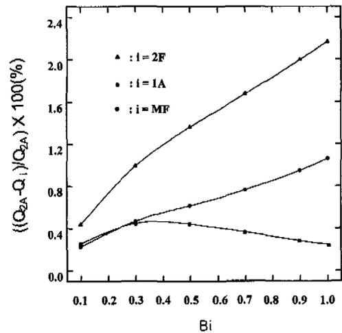
Fig. 4(a) The relative difference in the heat loss from the trapezoidal fin compared to the two-dimensional analytical method as a function of Biot number for  $L=1$ .
