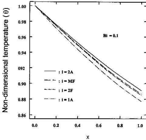
Fig. 5(b) The variation of the non-dimensional temperature at the fin center line (in the cases of two-dimensional analyses) along the x coordinate for  $L=1$  and  $Bi=0.1$ .
