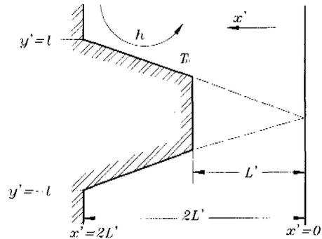
Fig. 1 Trapezoidal fin geometry used in the one-dimensional analysis.
