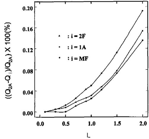
**Fig. 6(a)** The relative error in the heat loss from the trapezoidal fin compared to the two-dimensional analytical method as a function of  $L$  for  $Bi=0.01$ .
