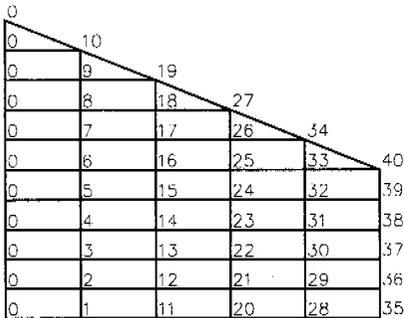
Fig. 3 Upper half fin geometry showing the 40 nodes in the finite difference method.
