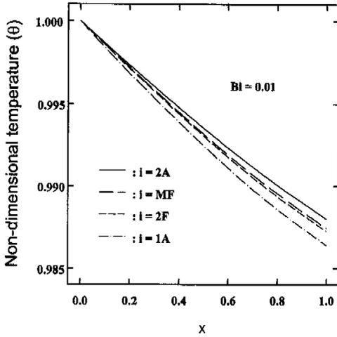
Fig. 5(a) The variation of the non-dimensional temperature at the fin center line (in the cases of two-dimensional analyses) along the x coordinate for  $L=1$  and  $Bi=0.01$ .
