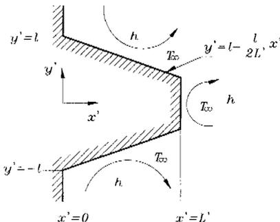
Fig. 2 Trapezoidal fin geometry used in the two-dimensional analysis.
