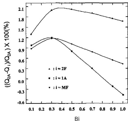
Fig. 4(b) The relative difference in the heat loss from the trapezoidal fin compared to the two-dimensional analytical method as a function of Biot number for  $L=2$ .
