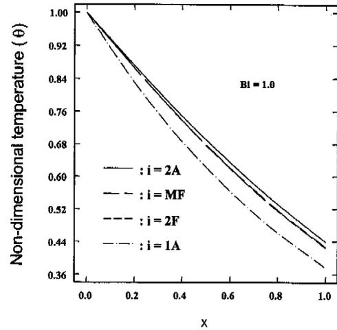
Fig. 5(c) The variation of the non-dimensional temperature at the fin center line (in the cases of two-dimensional analyses) along the x coordinate for  $L=1$  and  $Bi=1.0$ .
