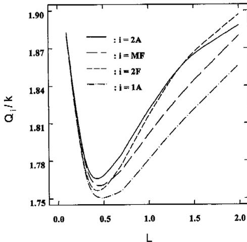
Fig. 7 The variation of the non-dimensional heat loss from the trapezoidal fin as a function of  $L$  for  $Bi=1.0$ .
