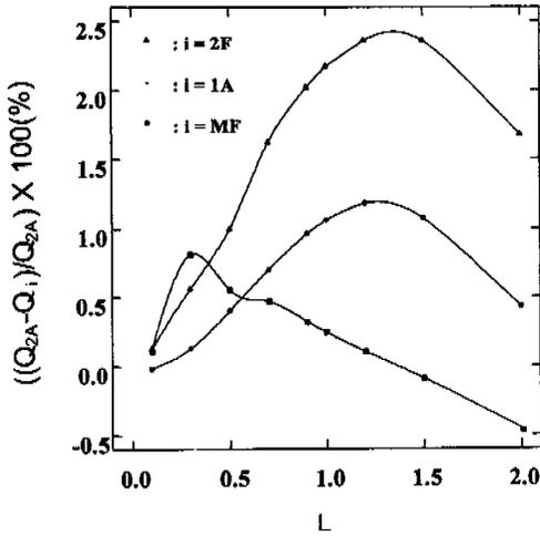
Fig. 6(c) The relative error in the heat loss from the trapezoidal fin compared to the two-dimensional analytical method as a function of  $L$  for  $Bi=1.0$ .
