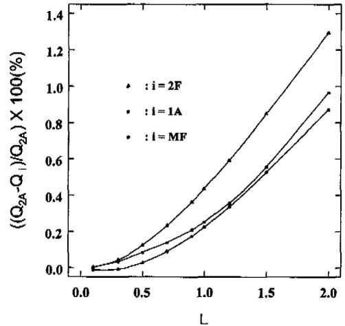
**Fig. 6(b)** The relative error in the heat loss from the trapezoidal fin compared to the two-dimensional analytical method as a function of  $L$  for  $Bi=0.1$ .
